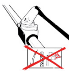
No welding, drilling etc.
