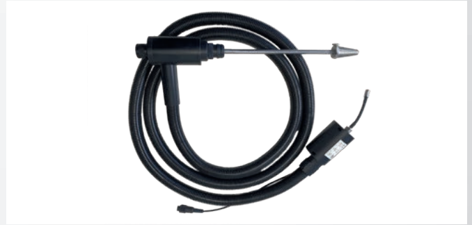
Heated gas sampling probe with heated sampling line, length 3 m, +130°C temperature regulated Gas temperature measurement using K-type thermocouple. With heated, easy replaceable quartz wool filter.
