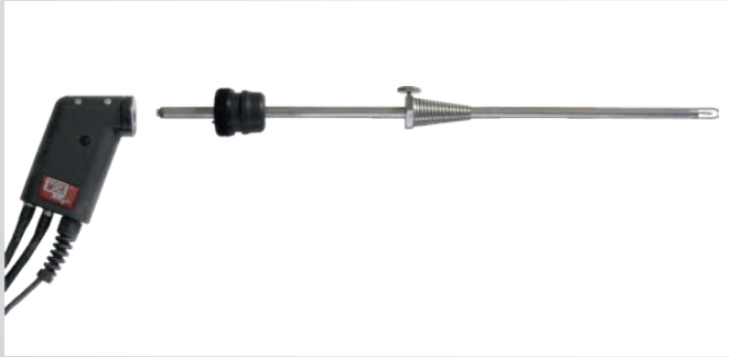
Gas sampling probe for industrial combustions, unheated, without filter for short, complete emission monitoring including NO 2 /SO 2 , probe handle for exchangeable tubes, with 2,7 m gas sampling line (VITON)
