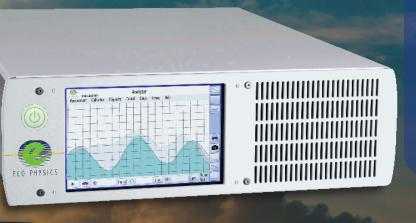
The nCLD  $EL^2$  is the next generation in two-channel NO/NO<sub>2</sub>/NO<sub>x</sub> measurement. Unique in speed and precision, the nCLD  $EL^2$  allows the continuous measurement of concentrations in the range of parts per million. Its new and intuitive user interface individually displays and connects to other instruments' data.
